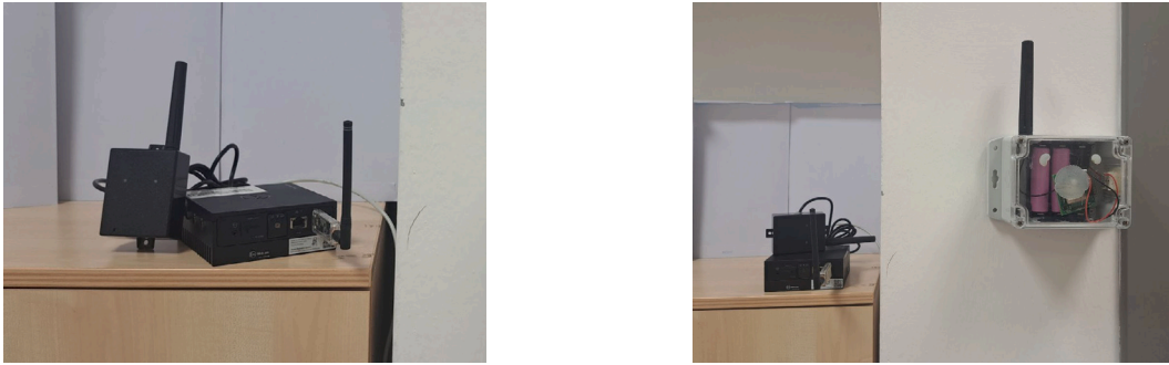
Fig. 5. Stationary Gateway on the left and Wireless Accelerometer on the right.
