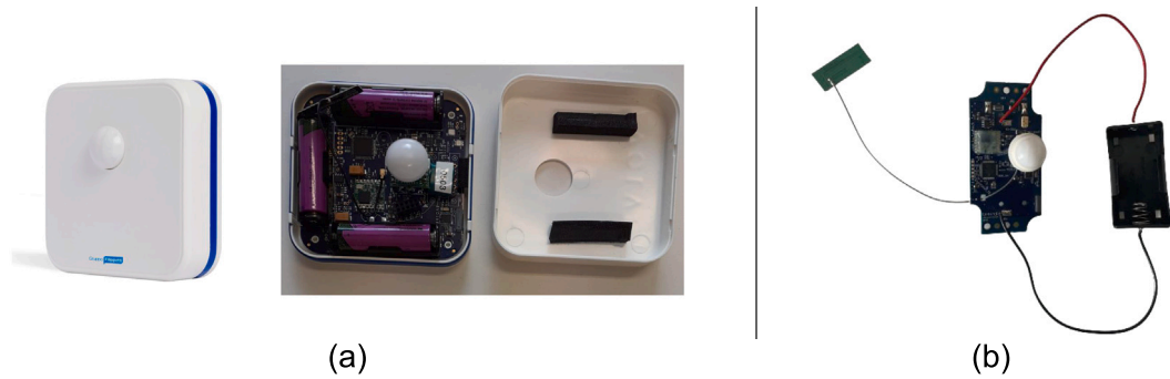
Fig. 4. The SAFE PIR. From the commercial version of the SmartNetwork PIR device (a) we defined the prototype of the SAFE PIR (b). The prototype provides a new modular layout that improves the integration in the SAFE furniture.
