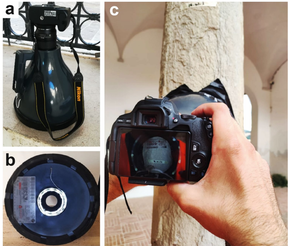
Fig. 5 Macro-photo tool employed in the sedimentological characterisation of the sandstone column: a bell-like cover with an external handle with camera placed on the narrower part of the tool; b LED lights inside the bell-like cover and transparent grain size scale pasted in the wider part of the tool; c application of the tool on the column, obtaining a high-quality picture (Fig. 6a, b) where to perform the grain size analysis
