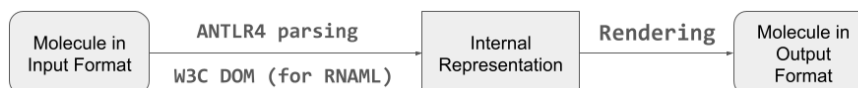
Figure 8. TARNAS workflow for translation. Each molecule file is parsed using either ANTLR4 or the W3C DOM, producing an internal representation of the secondary structure. This internal structure is then rendered in the requested output format.
