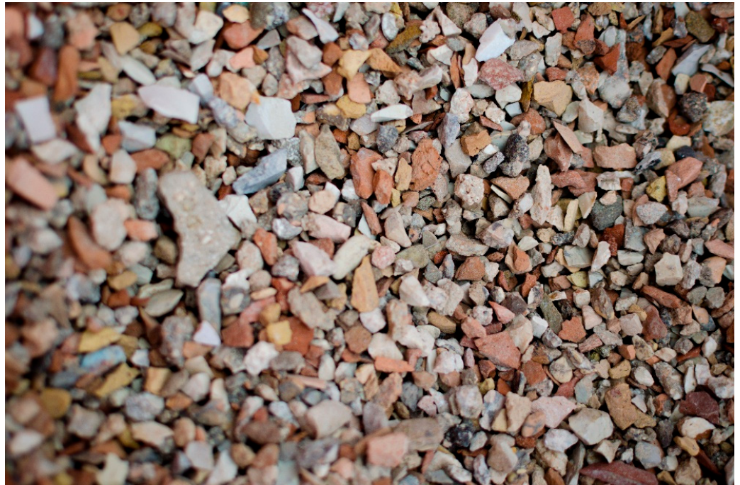
Figure 4. Recycled aggregates obtained from earthquake rubble in Central Italy, used as granular input for rubble-based printable mortars.
