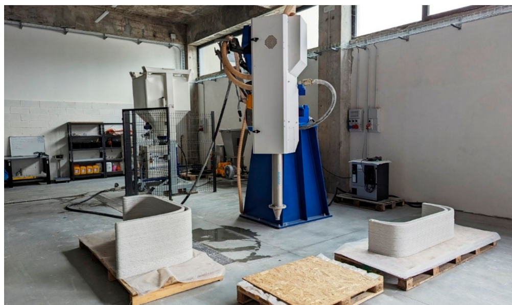
Figure 8. Robotic production cell used for the extrusion-based fabrication of rubble-derived components.
