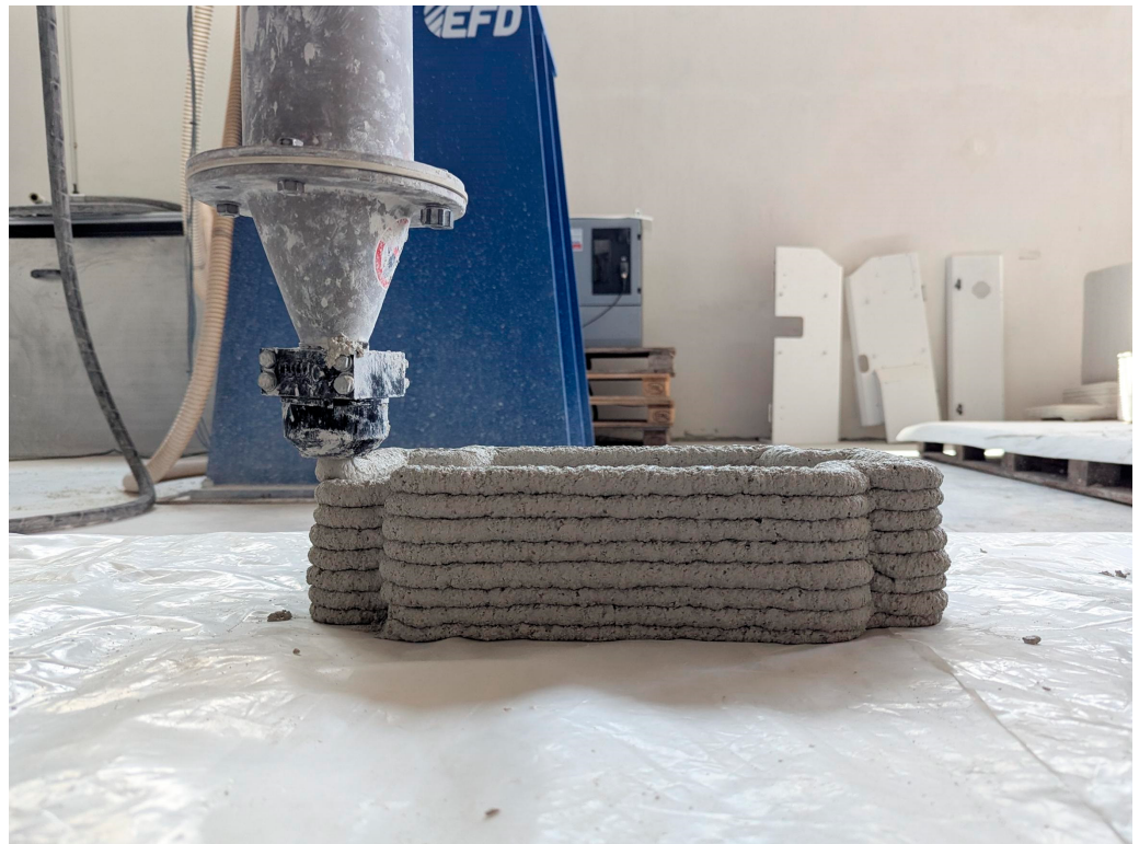
Figure 6. Robotic extrusion of a discrete block fabricated with a rubble-based printable mortar within the TRAP experimental setup.
