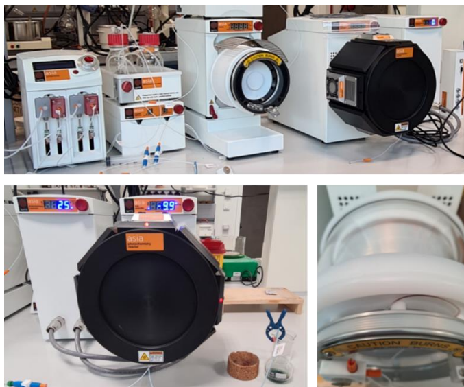
Figure 2.10 Asia Syrris equipment and flow set-up for \beta -nitroacrylates hydroalkylation
