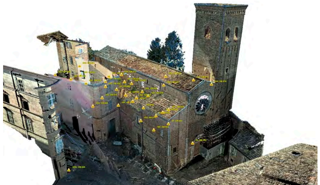
Figure 4. Point cloud with targets of the laser scanner and total station.
