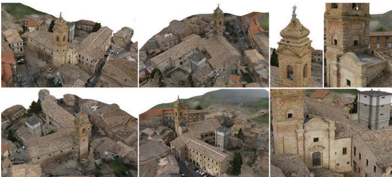
Figure 11. 3D mesh model obtained by merging LS and UAV data. Modelling: union of 865 surfaces into a single closed polysurface. Solid mesh and geometry (low number of polygons) for structural analysis.
