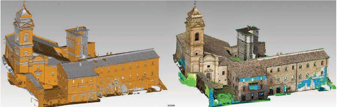
Figure 9. Best-fit alignment (reference length in red) of point clouds captured using UAV and TLS (tessellated using the 'Wrap' meshing algorithm).
