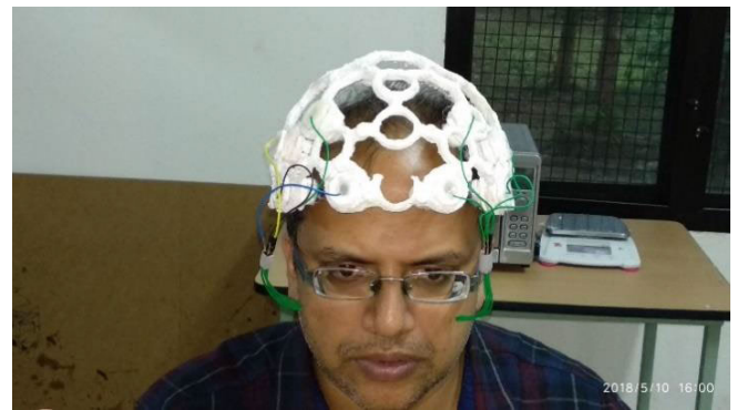
FIGURE 3. Signal acquisition using EEG sensor [21].
