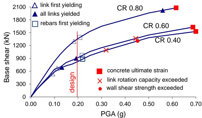
Figure 6. Results of multi-record nonlinear incremental dynamic analysis for a 6-storey HCW case study (results averaged over 30 accelerograms).
