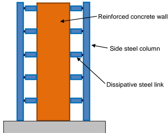
Figure 2. Innovative HCW proposed and tested.
