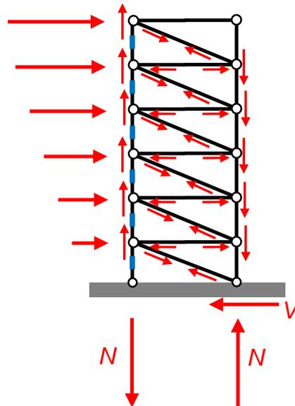
Figure 3. Static scheme of the considered SRCW system.
