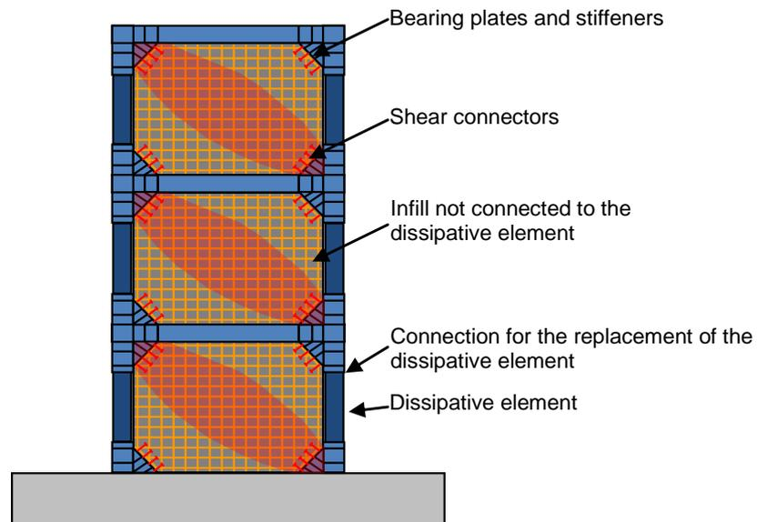
Figure 1. Innovative SRCW developed and tested.
