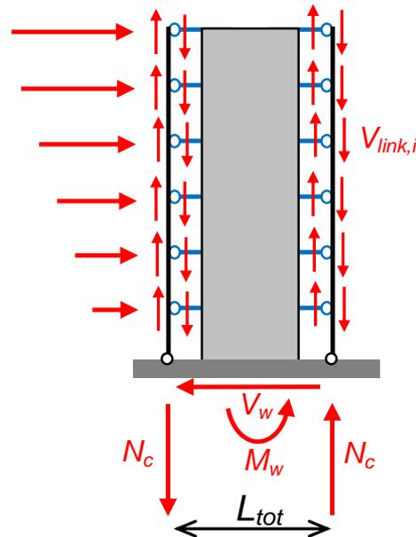
Figure 5. Static scheme of the considered HCW system.
