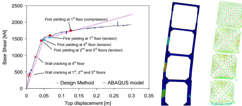
Figure 4. Comparison of pushover curves for SRCW and stress field in the steel frames and in the reinforced concrete wall.
