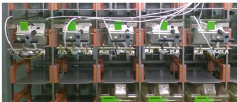
Figure 3.6: Video recording system on rack and DVC®Big Plate sensor.
