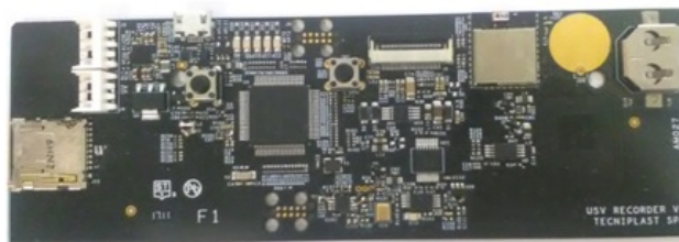
Figure 3.17: Tecniplast microphone module developed from MEMS microphone characterization and validation.
