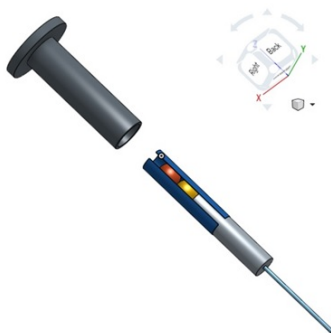
Figure 4.12: 3D drawing of the implantable optical system used.
