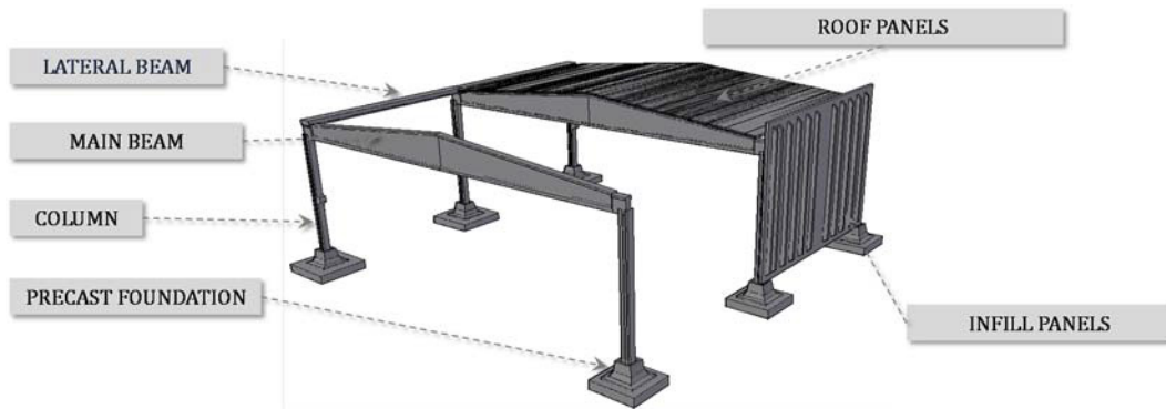
Figure 57: General scheme of r.c. precast building with indication of structural and non-structural elements.
