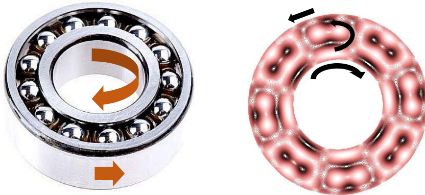
Figure 4: Ball bearing assembly (left). In the referring frame where the spheres are at rest, the internal and the external boundaries counter rotate, displaying different angular velocities. A similar effect can be achieved by solving the wave equation in a suitable annular region (right). In this circumstance, the size and the frequencies involved must be wisely calibrated.
