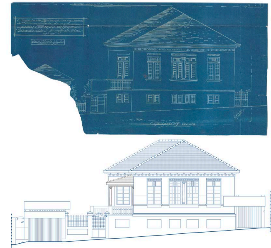
Fig.2 – Building in Rua Major Prado, 807 Jaú: graphical comparison of the design state from the blueprint available (source: Arquivo Municipal de Jaú) and the surveyed building in the year 2024. .
