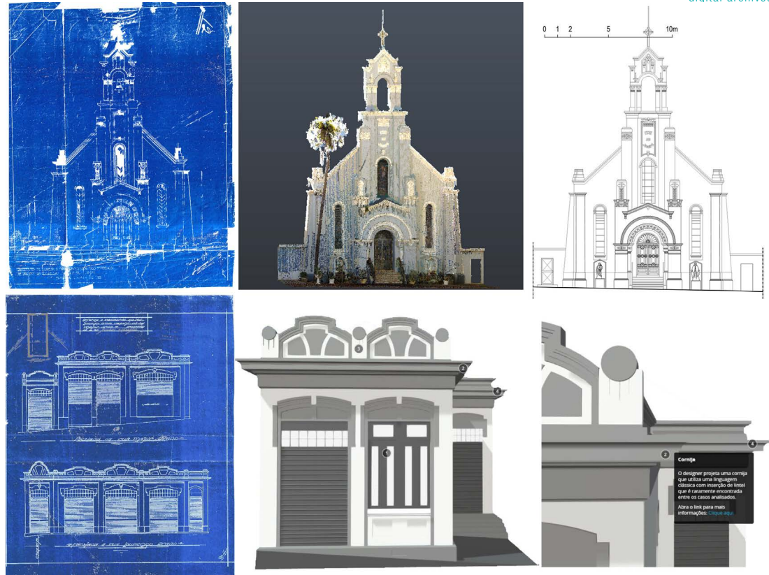
Fig.8 – From 2D Blueprint drawing to 2D and 3D digital model. On the top: Colégio San José (Jaú), blueprint (source: Arquivo Municipal de Jaú), 3D view from point cloud and 2D model of the main elevation. On the bottom: Building in Jaú, façade on Rua Major Prado and façade on Rua Lorenzo Prado Prado (drawing by Beppino Terrieri, source: Arquivo Municipal de Jaú), and 3D model for building analysis.
