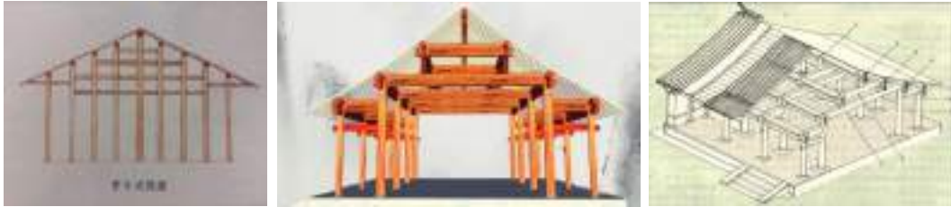
Figure 2.10 Through-Bucket Type; Lifting Beam Style; Well Dry Type 58
