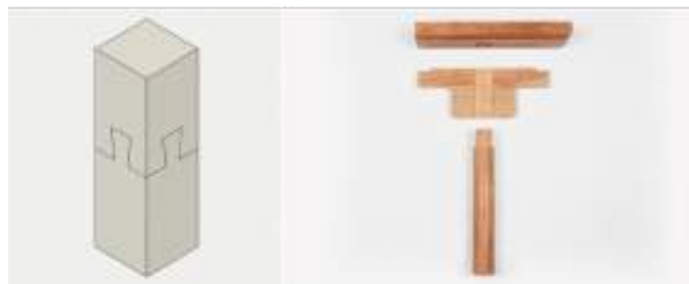
Figure 2.13 Mortise and Tenon Types 62
