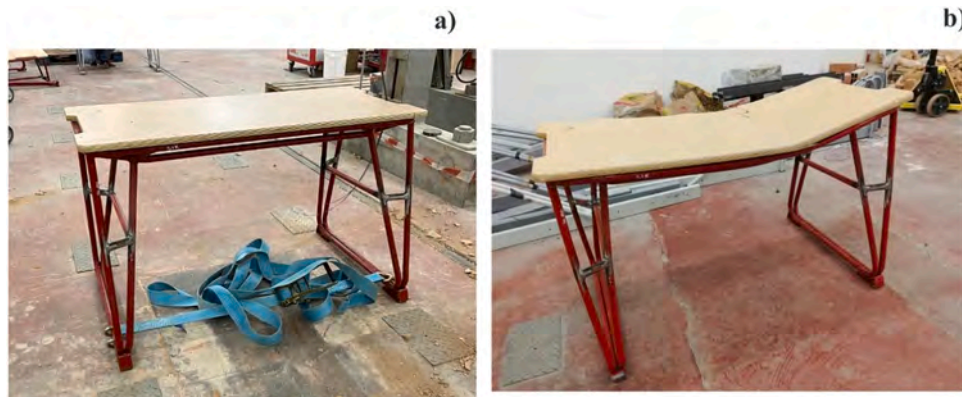
Fig. 20. Impact test performed with a floor portion of 600 kg: a) test setup with ratchet belt; b) the prototype after the impact.
