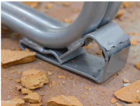
Fig. 15. Proposed dissipative foot collapsed after the loading test.
