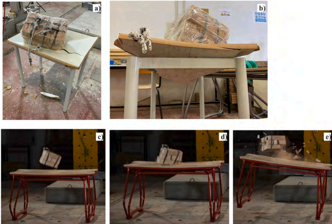
Fig. 19. Impact test performed with a floor portion of 36 kg: a) traditional desk tabletop breach; b) traditional desk tabletop-frame separation; c) impact on the life-saving desk; d) with energy dissipation; e) and overall bouncing.
