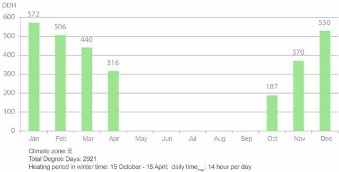
Fig. 8 Climate data related to the monthly heating degrees days in Terracino; elaborated by calculating the ratio between the total Heating Degree Days of Accumoli (2921 HDD) and the sum of the Heating Degree Hours recorded by the Weather Tool for the months during which heating is legally mandated.
