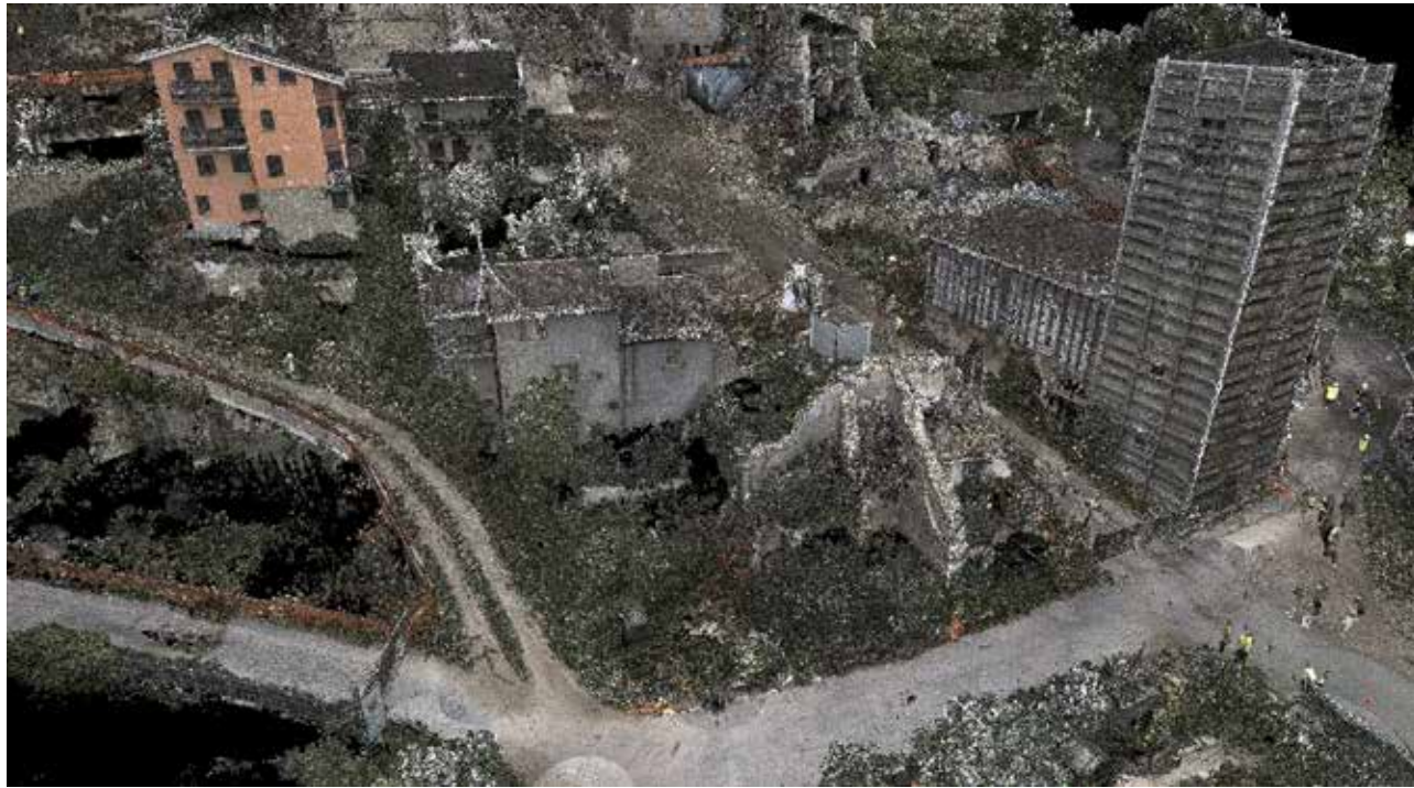
Fig. 4 3D laser scan point cloud region showing the center of Accumoli including the city tower and nearby buildings and ruins. The scans also show artifacts caused by people crossing the line of sight of the scanner. Such artifacts can be removed in post-processing..
