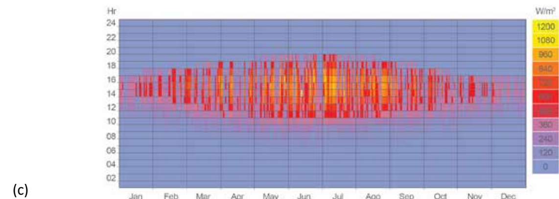
Fig. 13 (a) Plan of the analysis of the azimuthal orientation of the exposed roofs in the building stock. (b) Calculation of the available irradiated roof portions and the incident solar radiation during the winter season, the summer season and the annual total values, according to the different azimuthal orientation. (c) Graphic overview of the annual incident direct and diffused solar radiation for the different azimuthal oriented roof portions.
