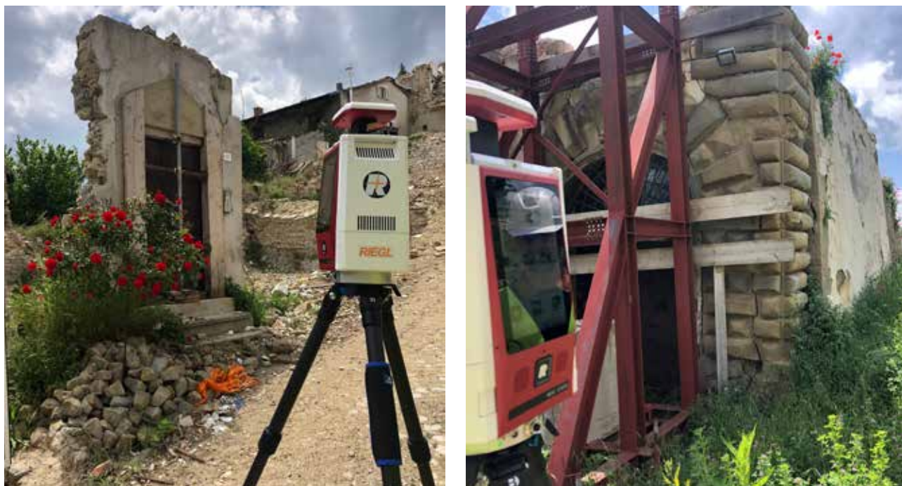
Fig. 2 Scanning in a position in gravelled alleys and other areas almost completely reclaimed by nature. Scanning is possible as long as the scanner and the optional tripod can be set up stably. The distances between the scan positions are chosen based on the geometric complexity of the environment and typically range between 5 and 15 meters.
