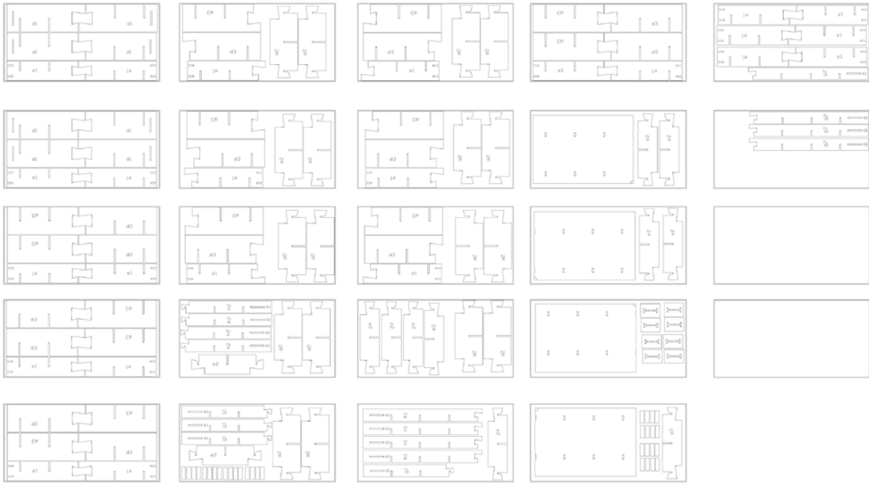
Fig. 5 Nested pieces in the plywood board prepared for cutting. (Image by the Authors).
