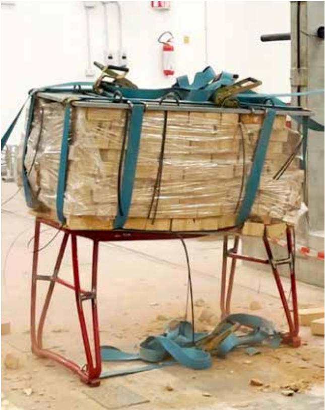
Fig. 6 Experimental verification of the protection capacity of a life-saving school desk under impact simulating structural collapse.
