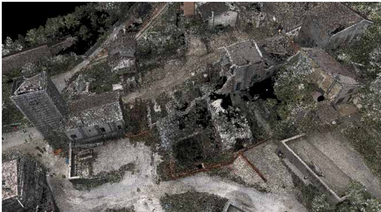
Fig. 5 Oblique view of the city center and tower from a virtual viewpoint. This view clearly shows that it was not possible to cover all roofs, courtyards, and interior rooms of destroyed building from safe terrestrial scanning positions. Some of the missing data could be supplemented by airborne laser scanning or image-based modeling.
