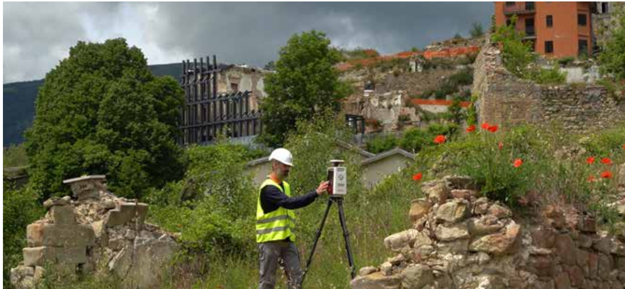
Fig. 1 Laser scanning in Accumoli using the Riegl VZ600i. This scanner is much faster than previous models, allowing up to 60 scans per hour. This is mainly due to the possibility of moving it from one scan position to the next one very quickly, because of its lightweight construction and possibility of markerless operation.
