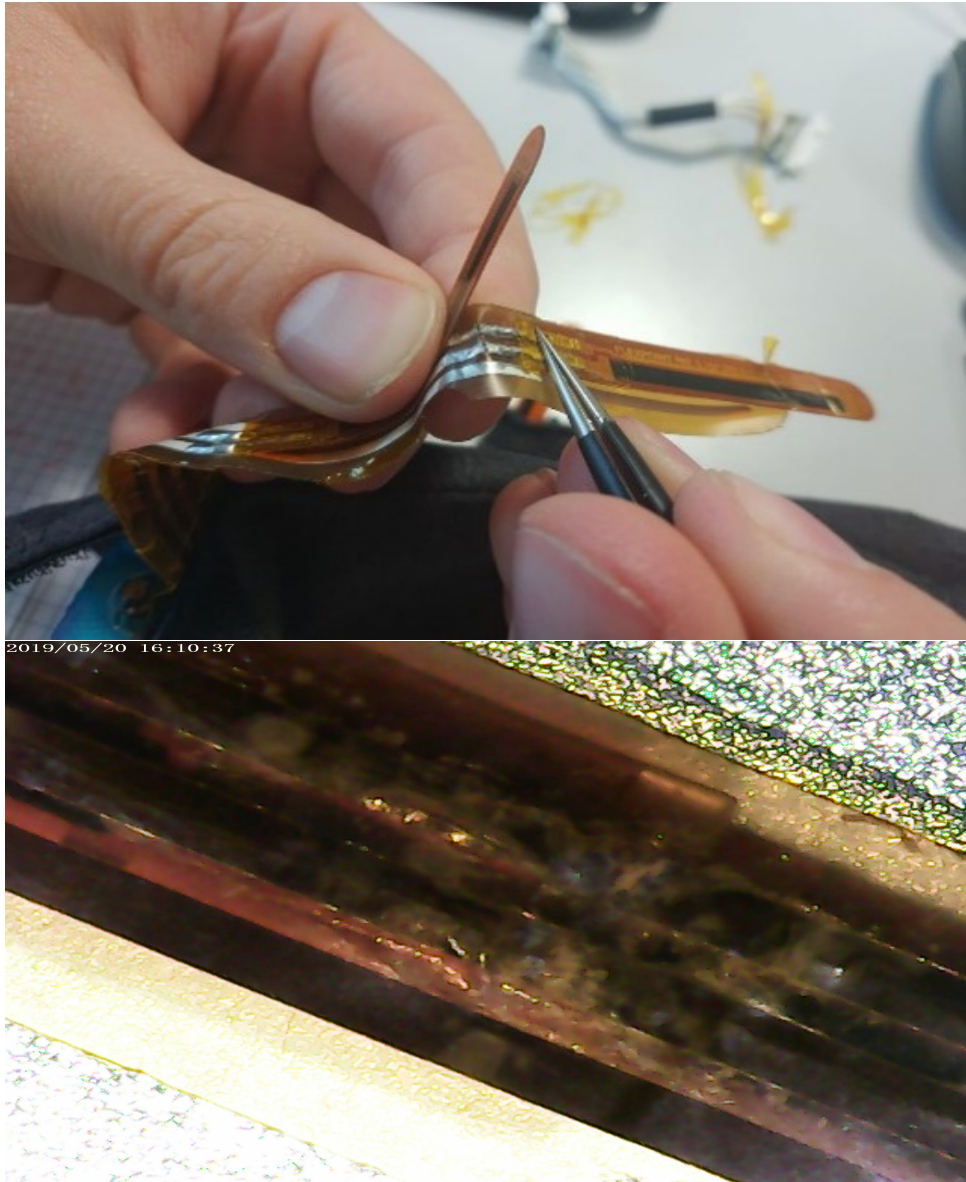
FIGURE 5.1: Broken F-PCB's tracks after few hours incorrect usage, flex sensor's pin has been stressed during usage, white surface means broken bus
