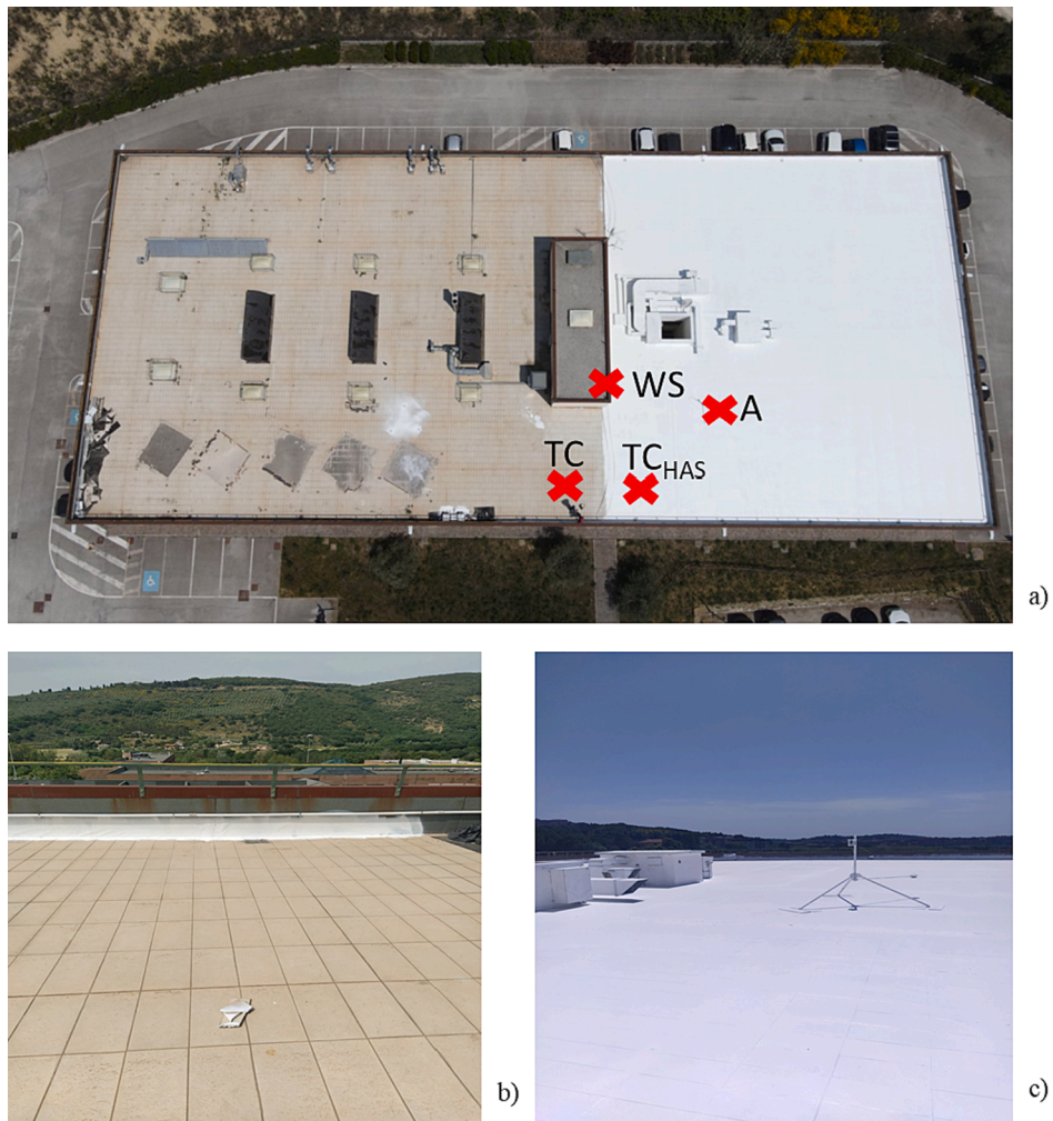
Fig. 2. An aerial view of the test facility at CIRIAF (University of Perugia) with the shape of the equipment (i.e. A, WS, TC, and TC HAS ) evidenced in red (Fig. 1a); surface under test before albedo change (Fig. 1b); surface under test after albedo change (Fig. 1c). (For interpretation of the references to color in this figure legend, the reader is referred to the web version of this article.)
