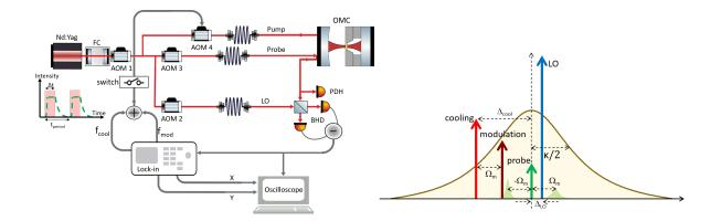
FIG. 2: Layout of the experimental setup (see text) and conceptual scheme of the field frequencies. The LO is placed on the blue side of the probe and detuned by  $\Delta_{\text{LO}} \ll \Omega_{\text{m}}$ , therefore the Stokes line is on the red side of the LO, while the anti-Stokes line is on its blue side. In the heterodyne spectra, they are located respectively at  $\Omega_{\text{m}} + \Delta_{\text{LO}}$  (Stokes) and  $\Omega_{\text{m}} - \Delta_{\text{LO}}$  (anti-Stokes).
