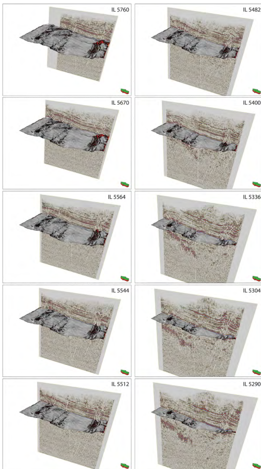
Figure 7. Vertical sections (inlines; IL) through the 3D seismic volume, showing east (upper left) to west (lower right diagram) development of structures. The spacing between adjacent sections is variable (in the range of 210–1,590 m; for reference, the IL spacing is 15 m). Top Muschelkalk surface with overlying variance attribute obtained by seismic interpretation is also shown.
