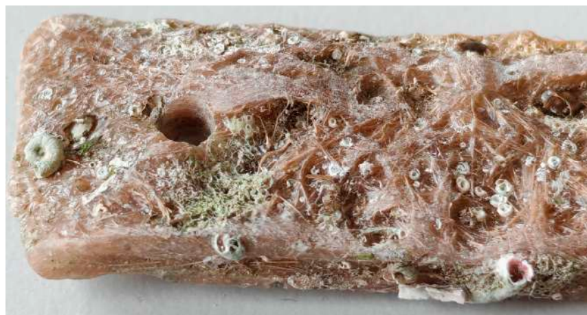
Figure 3. Composite specimen after seawater exposure at a 2 m depth: the drilled hole for insertion into the carousel is shown on the left.
