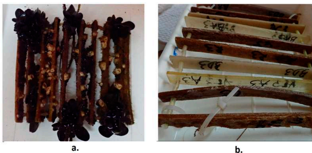
Figure 5. Test samples after six months of exposure: (a) samples retrieved from 0.5 m depth (Site 2), showing fouling communities; (b) samples from the splash zone (Site 3), with no fouling development due to desiccation and high temperature.
