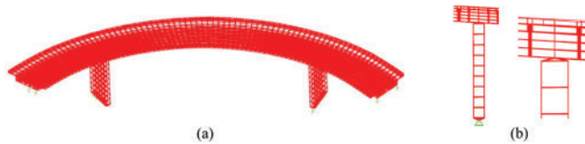
Figure 6. Numerical model of the case study bridge: (a) global view; (b) details of piers modeling
