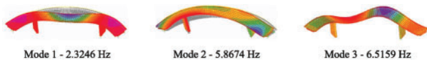
Figure 12. Mode shapes and natural frequencies obtained from the numerical model simulating the actual structural response of the bridge
