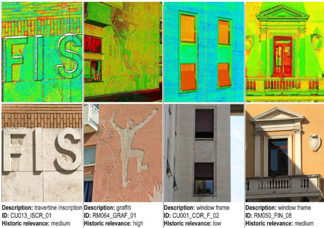
Figure 14. Examples of distinctive elements and their description, codification, and historic relevance: ( top line ) point cloud reflectance visualization; ( bottom line ) pictures of the corresponding images.
