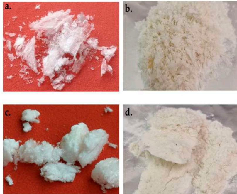
Figure 4. Result of keratin extraction: extracted keratin (a) and residue (b) from chicken feathers; extracted keratin (c) and residue (d) from sheep wool.
