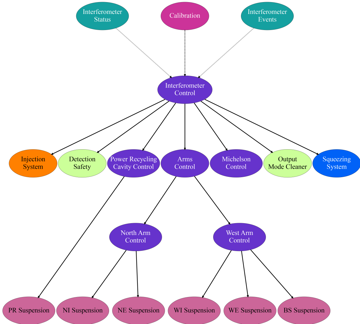
Figure 3. Metatron nodes hierarchy used during the O3 run.
