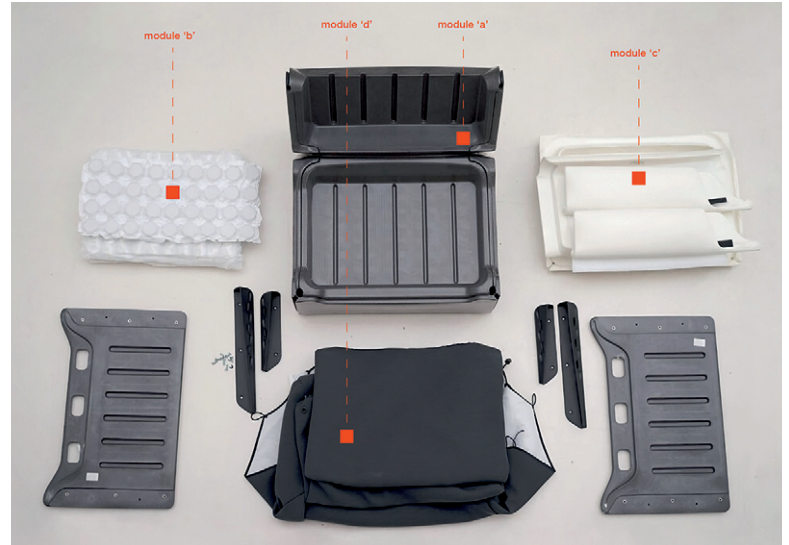
Fig. 7, 8 | Costume Armchair and main modules of the Armchair version: the armchair core 'a'; the seat, composed of a spring insert 'b' and a polyurethane layer 'c'; the fabric cover 'd' (credit: Magis).
