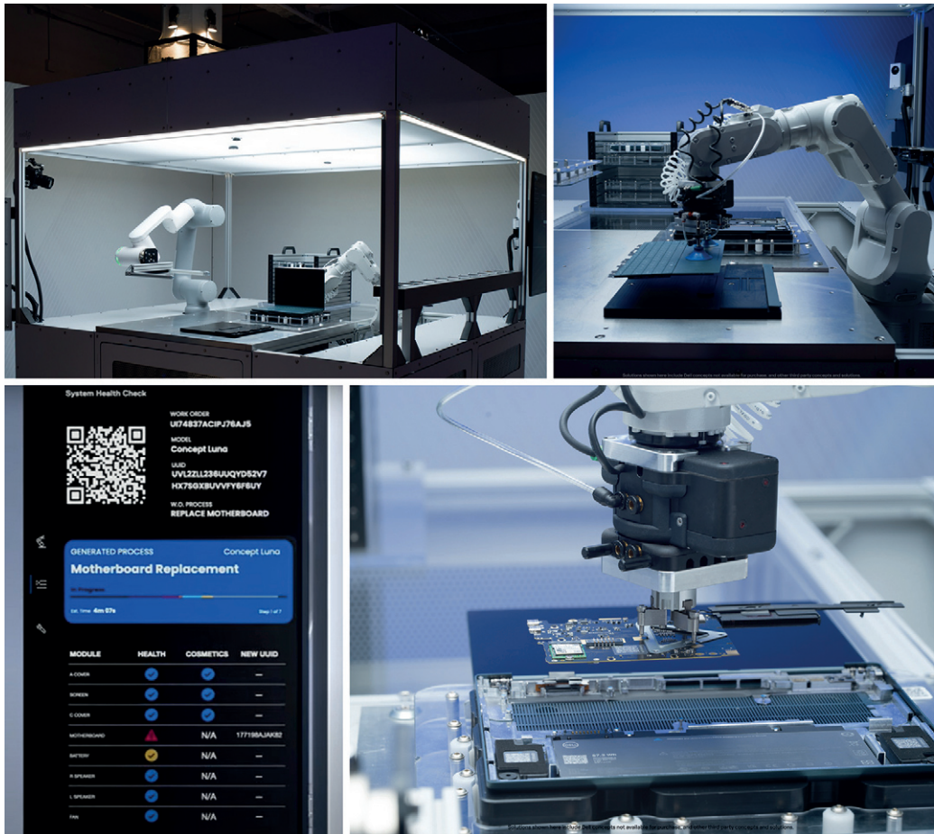
Fig. 14 | Some stages of the Luna notebook assembly process using robots and telemetry to diagnose the health of individual components within the 'micro-factory' (credit: Dell Inc.).
