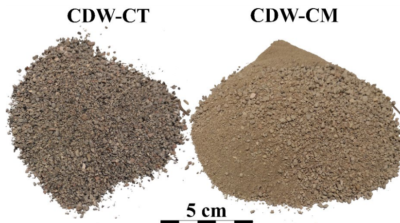
Figure 1. CDW samples at the end of the grain-size standardisation procedure in accordance to EN 196-1: CDW-CT on the (left); CDW-CM on the (right).
