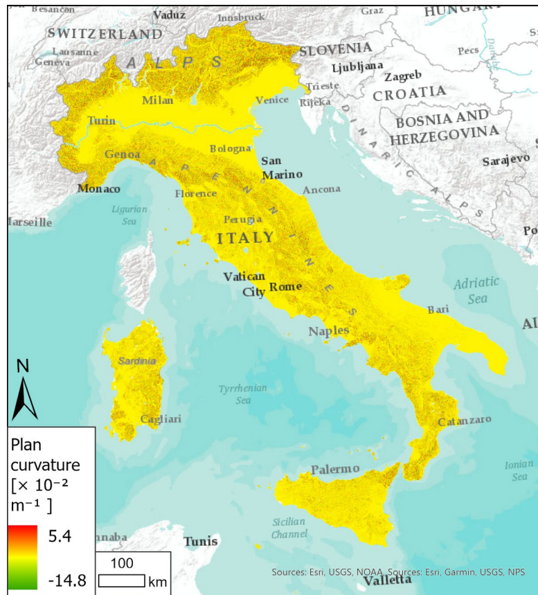
Figure 34. Plan curvature was calculated with a spatial resolution of 150m. The raster has a minimum value of -14.8 \times 10^{-2} m^{-1} , a maximum value of 5.3 \times 10^{-2} m^{-1} , an average value of 0.005 \times 10^{-2} m^{-1} and a standard deviation of 0.15 \times 10^{-2} m^{-1}
