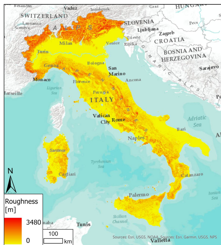
Figure 29. Roughness with a spatial resolution of 150m. The raster has a minimum value of 0, a maximum value of 3480, and an average value of 74
