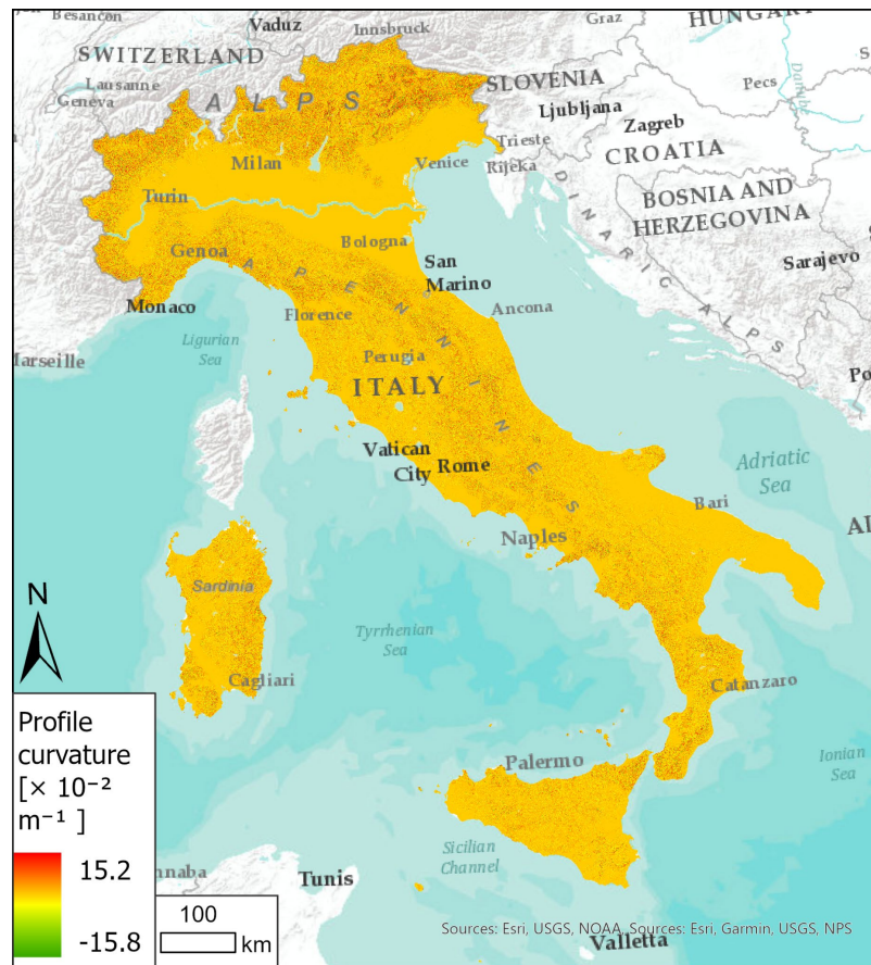
Figure 33. Profile curvature was calculated with a spatial resolution of 150m. The raster has a minimum value of -15.8 \times 10^{-2} \text{ m}^{-1} , a maximum value of 15.2 \times 10^{-2} \text{ m}^{-1} , an average value of 0.005 \times 10^{-2} \text{ m}^{-1} and a standard deviation of 0.13 \times 10^{-2} \text{ m}^{-1}
