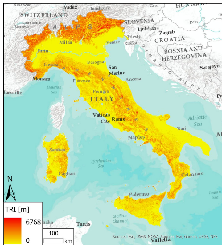
Figure 31. TRI map calculated with a spatial resolution of 150m. The raster has a minimum value of 0, a maximum value of 6768m, and an average value of 78m
