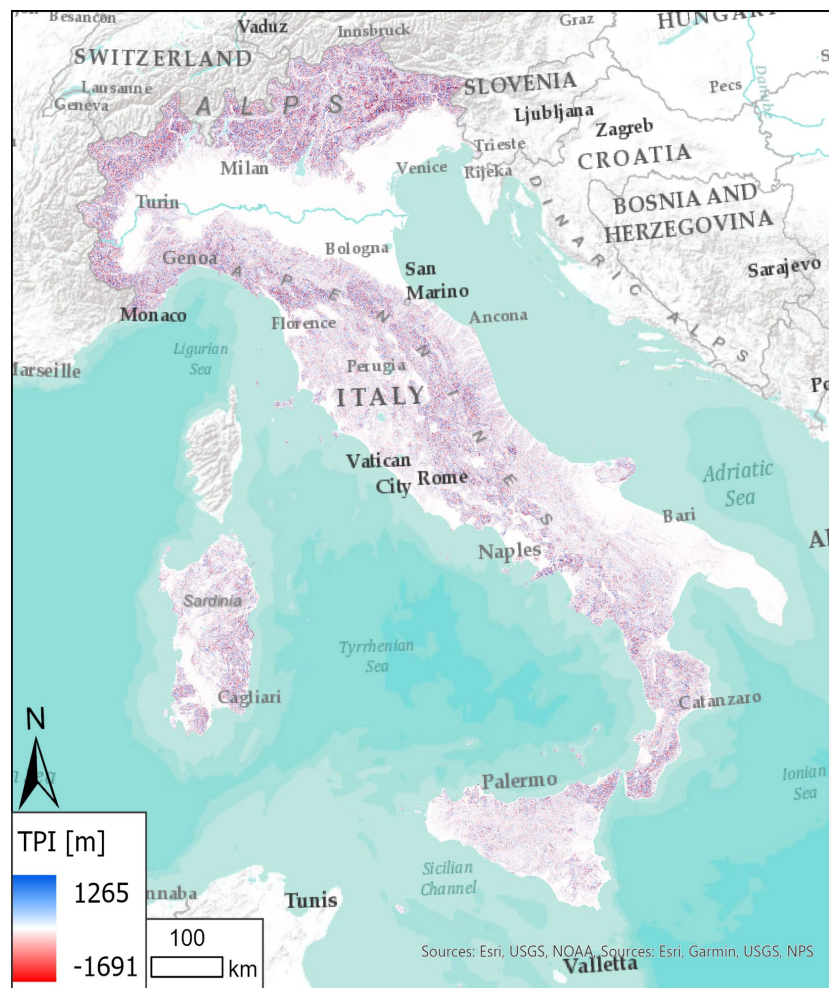
Figure 32. TPI map calculated with a spatial resolution of 150m. The raster has a minimum value of -1691m, a maximum value of 1265m, and an average value of 2.52m
