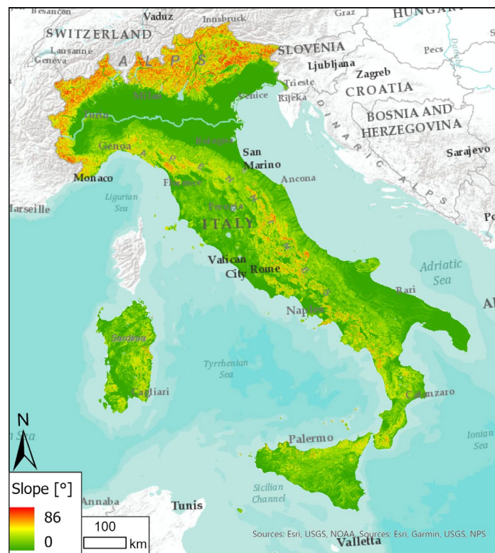
Figure 28. Map of slopes expressed in degrees and calculated with a spatial resolution of 150m. The minimum value is 0°, the maximum value is 86°, and the average value is 9.4°
