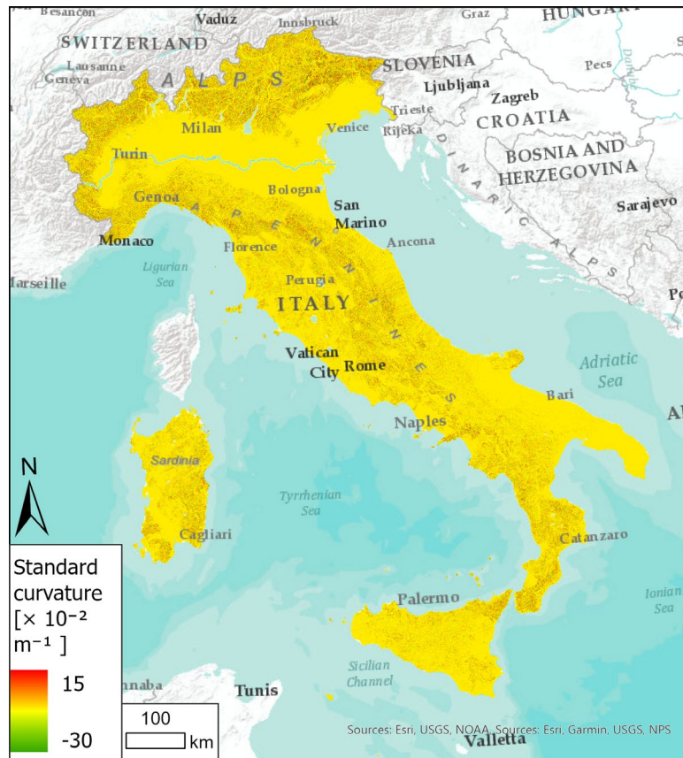
Figure 35. Standard curvature was calculated with a spatial resolution of 150m. The raster has a minimum value of -30 \times 10^{-2} \text{ m}^{-1} , a maximum value of 15.3 \times 10^{-2} \text{ m}^{-1} , an average value of -8.4 \times 10^{-16} \text{ m}^{-1} and a standard deviation of 0.25 \times 10^{-2} \text{ m}^{-1}
