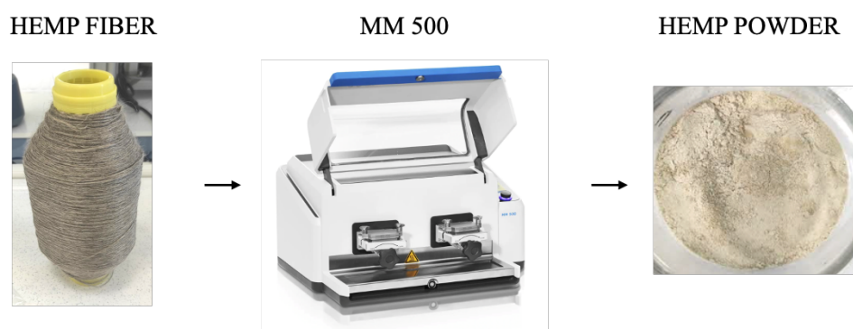
Figure 2.22. Grinding of hemp fibers with MM 500 nano mill
