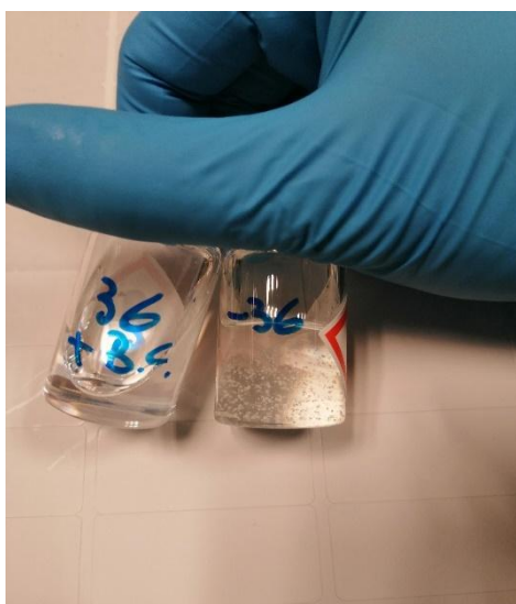
Figure 73. Gelation results on 36+Benzoyl Chloride (no gel, left) and 36 (gel, right)
