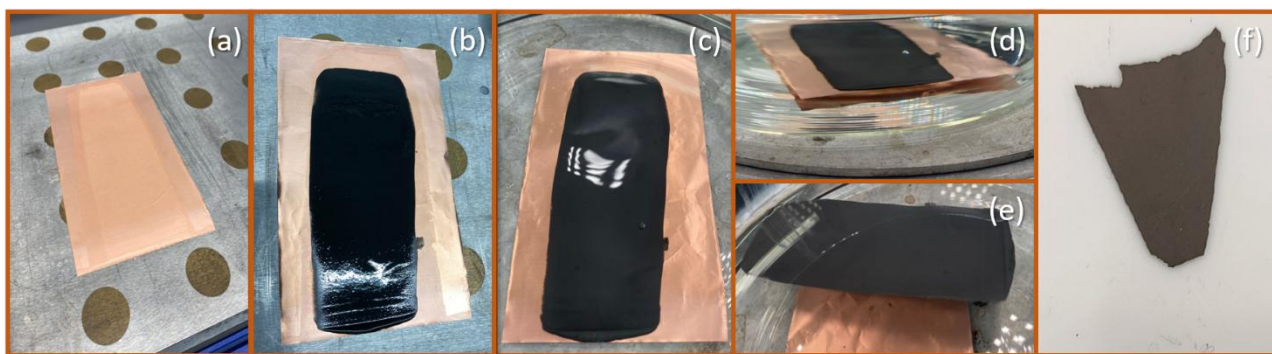
Figure 2.25: Photographic images of LFMP_SS electrodes during casting procedure: (a) coating of a thin layer of CMC solution onto a copper foil; (b) coating of PVdF-based layer onto the dried CMC film; (c-e) immersion of the coating in water and subsequent dissolution of the CMC layer; (f) final LFMP_SS electrodes.
