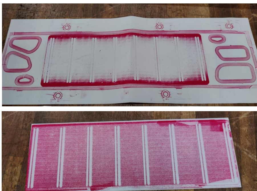
Fig. 6.5 Fuji film pressed with the gaskets and without gaskets
