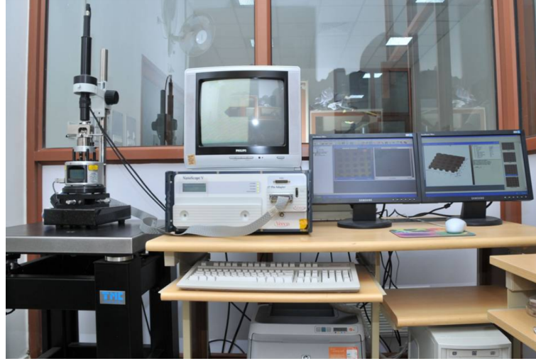
Figure 2.2: Atomic Force Microscopy set up from Veeco Instruments, present in the CSIR- National physical laboratory, New Delhi, India.
