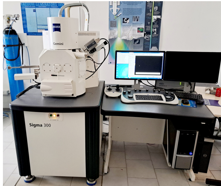
Figure 2.8: Field Emission Scanning Electron Microscopy system from ZEISS SIGMA 300, at the facility of Department of Physics, UNICAM.
