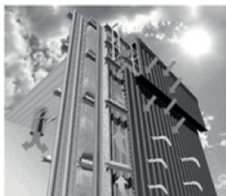
Combined solar thermal and PV envelope component
