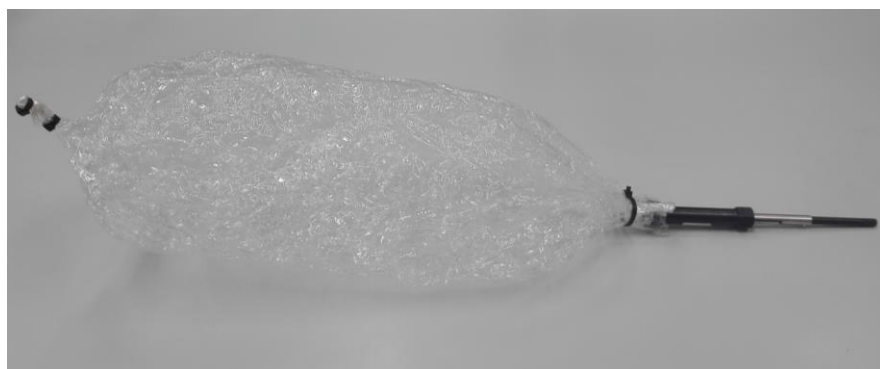
Figure 26. New system of extraction: SPME fiber inserted inside the cut vial, through a pierceable septum
