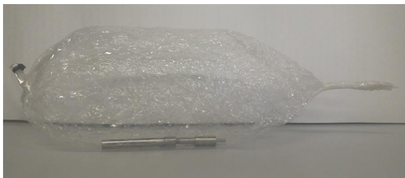
Figure 22b. System used to perform extraction with SPME fiber exposed inside the bag
