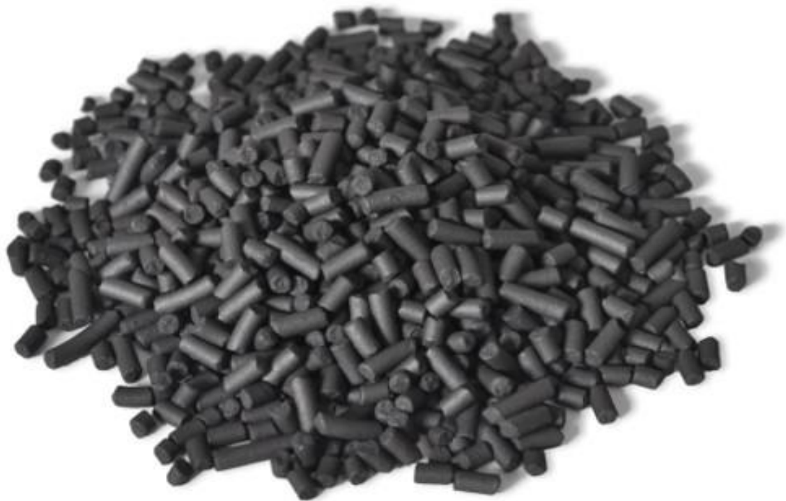
Figure 15. Granules activated charcoal (GAC)
