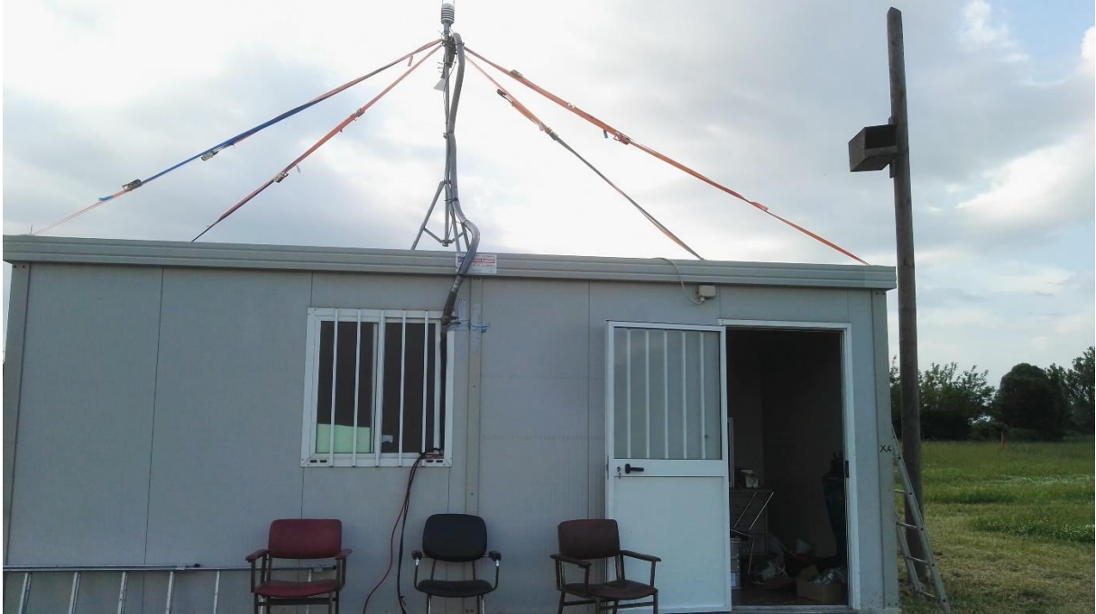
Figure 5.5: Container for the measurement apparatus. At the top of the container, the weather station and the sampling line.
