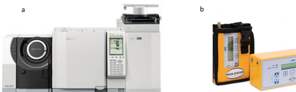
Figure 2.1: a) TD-GC-MS used for BVOC analysis; b) Sampling pumps.
