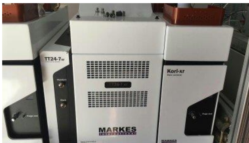
Figure 5.7: On-line thermal desorption (TT24-7) and accessories to remove the humidity (Kori-xr).
