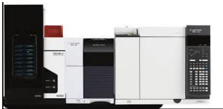
Figure 4.3: TD-GC-TOF-MS instrument used for BVOCs analysis in Max Planck Institute for Chemistry (MPIC).
