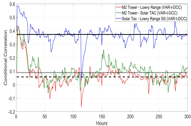
Figure 13: Cross-site correlation obtained with the VAR-t-DCC model for the the three pairs of sites.
